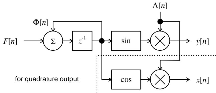
Figure 7.5 The Phase-Accumulator Oscillator
